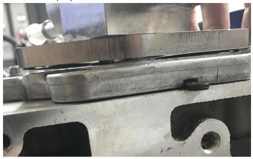
If there is no preload, install the 0.080" lash cap. You will want to achieve maximum preload so the lifter stays on the cam-lobe at all rpm (no float). A good pre-load would be 0.5-0.58mm (0.020-0.025").
