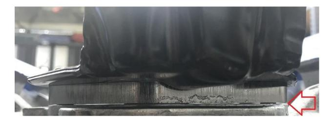
However if the fuel pump drive rod does bottom out before the bolts are tight, with no gasket, while the fuel pump lobe is at full lift (see picture), you will destroy the pump if the engine is ran this way.
