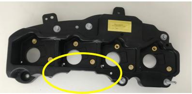
7. Install coil cover according to this picture. If coil cover touches Pump outlet fitting, some more cutting or grinding might be needed. Do not force it down with the bolts, it will crack.
