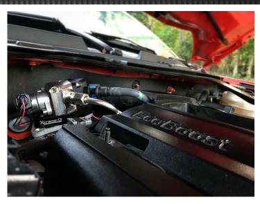
This GDI high pressure pump was developed to replace the Bosch OEM high pressure pump. It delivers up to 35% more fuel flow when mounted on the same CAM-Lobe.
